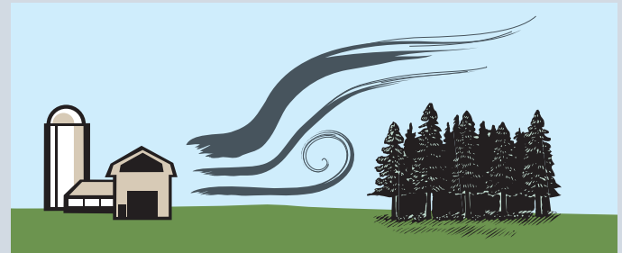
Figure 2: Trees can dissipate odor by forcing the plume to elevate and stir.
